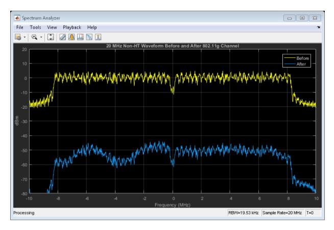
The free-space path loss accounts for the approximately 50 dB of separation between the waveform before and after it passes through the 802.11g channel.
