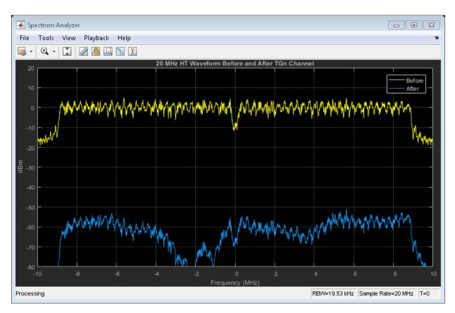
The path loss results from the default transmitter-to-receiver distance of three meters, and from shadowing effects. This path loss accounts for the roughly 50 to 60 dB of separation between the waveform before and after passing through the TGn channel. The frequency selectivity of the delay profile is seen in the signal level variation across the frequency spectrum.
