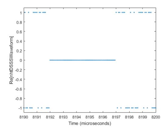
Sample values in DSSS modulation are -1 or 1. The plot shows the real values for a section of the waveform that includes the tail end of packet one, the 5 microsecond idle period, and beginning of packet two for the non-HT format DSSS modulated waveform.
