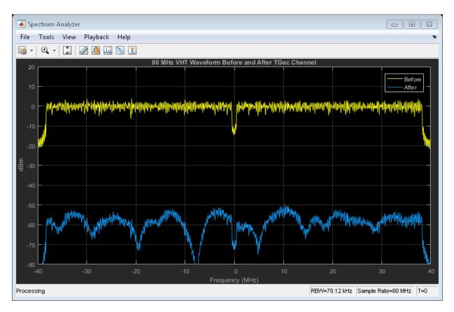
The path loss results from the default transmitter-to-receiver distance of three meters, and from shadowing effects. This path loss accounts for the roughly 50 to 60 dB of separation between the waveform before and after passing through the TGac channel. The frequency selectivity of the delay profile is seen in the signal level variation across the frequency spectrum.
